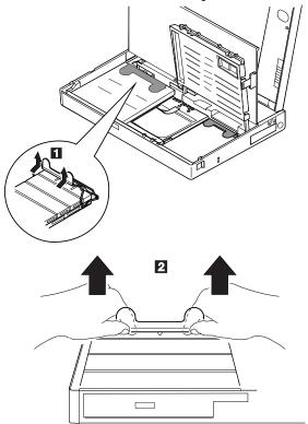
**Warning:** When replacing the CD-ROM/diskette drive, check that the standby battery is seated correctly to prevent damage to the drive.
